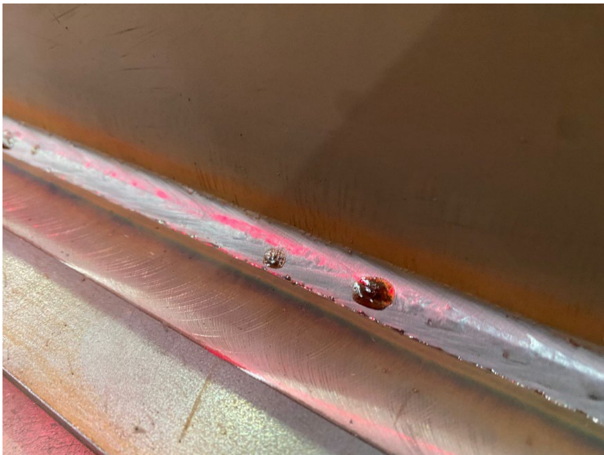
Mantis® produces high quality welds. This 6.5mm 2F weld was produced at 90cm/min travel speed (10mm 350MPa mild steel / 1.2mm ER70S6 80/20Ar/CO2 Twin).
