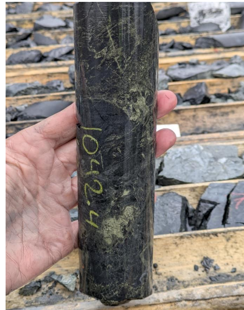
Image: Tillex Project TX26-010 drill core at 74.4m, disseminated, fracture fill and coarse chalcopyrite within argillite
