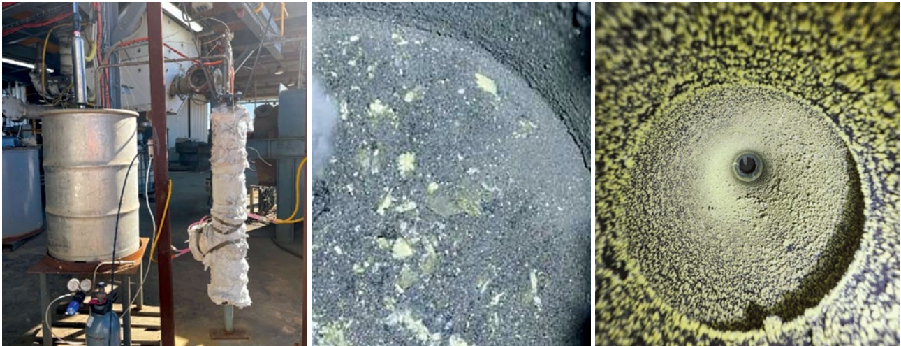
Figure 3 (L-R) – Vertical kiln prototypes, pyrrhotite product after pyrite conversion and sulphur collection in condenser
