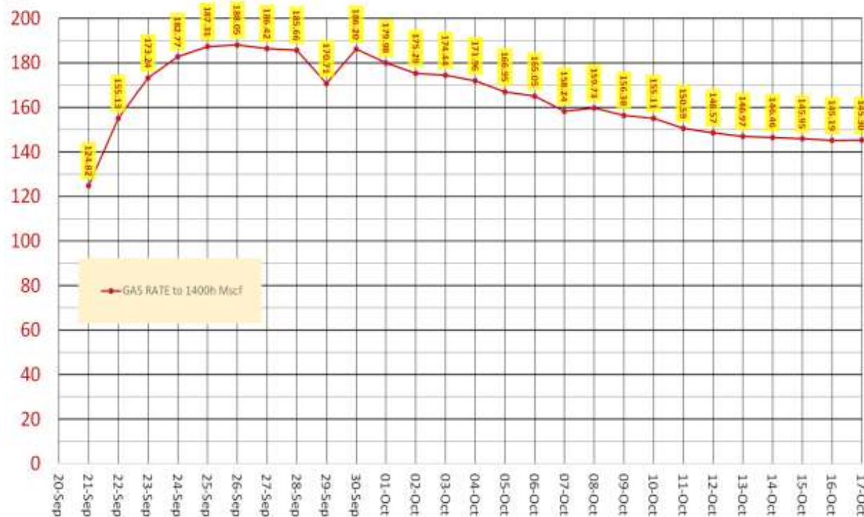
Figure 4 – Production test well 271-KA03PT06 daily gas flow rate. The volume recovered during 27 days of continuous testing was 4,432 Mscf of approximately 98.5% methane.
