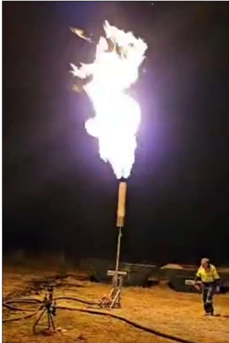
Figure 3 – Production test well 271-KA03PT06 being choke tested.
