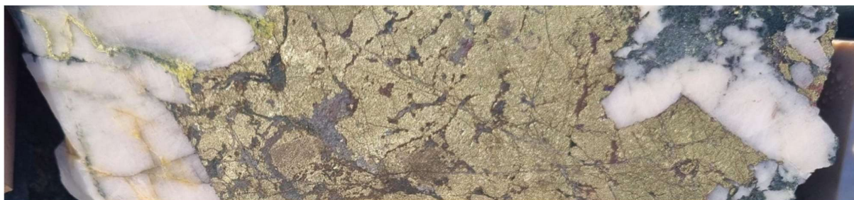
Figure 10: GGDD004 82.30 – 82.50m Brecciated quartz – magnetite UST textures with massive broken chalcopyrite with trace bornite. The associated sample interval 81.87m – 82.81m returned 8.46% Cu, 0.59g/t Au, 25g/t Mo.
