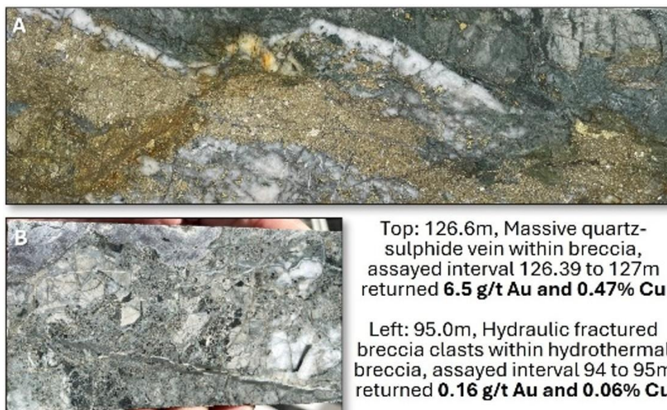
Figure 3. Examples of hydrothermal brecciation as seen in EB001
