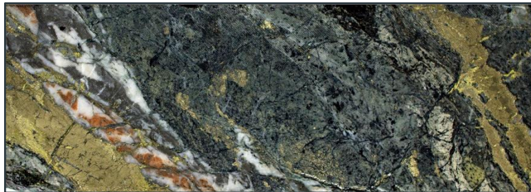
SPRCD037 @ 436-437m 11.6g/t Au. Massive sulphide veins
