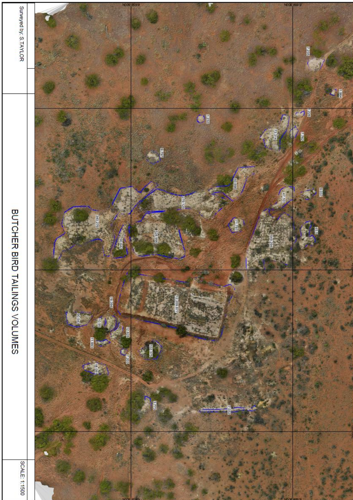
Figure 4 Outline of 3D shapes and volumes generated by UAV Lidar at the Butcher Bird Tails at Marda Central
