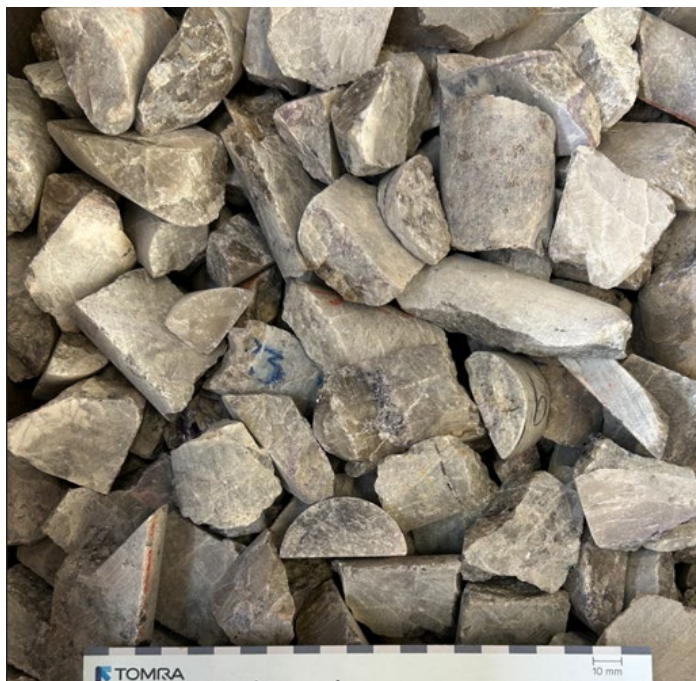
Figure 1: Pollucite concentrate (~12% \text{Cs}_2\text{O} ) produced from prior XRT ore sorting program (see news release dated October 9, 2025), of which a portion was used as feed for the bench-scale caesium extraction and recovery program through Koch Technology Solutions discussed herein.
