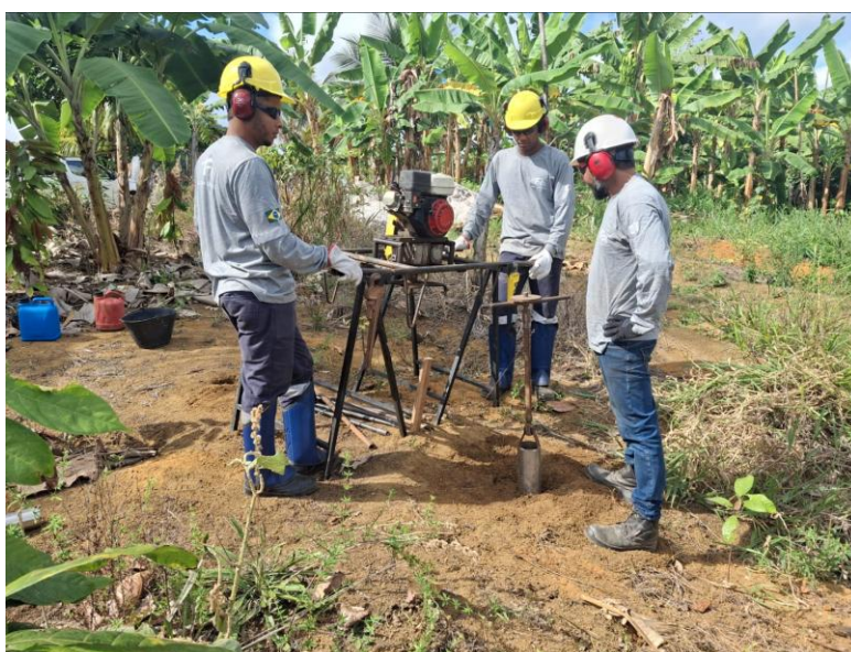
Figure 3: Mechanised auger drilling at the NE Target, Campo Grande Project.
