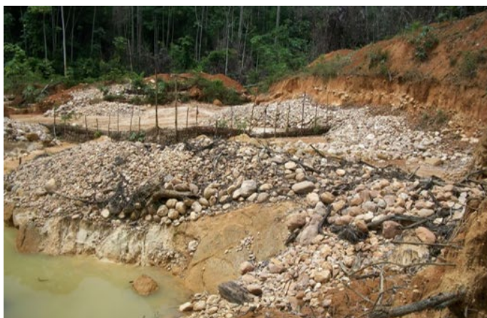
Figure 6 – Artisanal pit workings on the Gonini Project [circa 2019] (left) pit in saprolite exposing coarse quartz-rich gravels; (right) small-scale pump-and-sluice operation on the pit floor.
