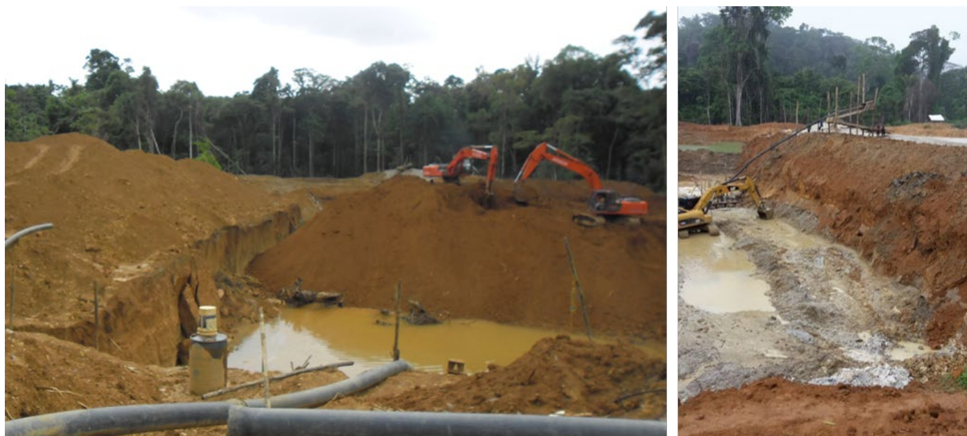
Figure 4 – Excavator-assisted workings on the Gonini Project [circa 2020]: (left) pit wall exposing the weathering profile from lateritic cover into saprolite; (right) excavator feeding a sluice at the pit face.
