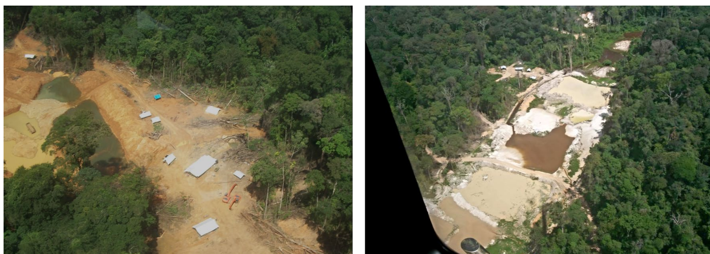
Figure 5 – Aerial view of active artisanal workings on the Gonini Project [circa 2020], showing cleared alluvial flats, settling ponds and camp infrastructure within the forested Sara Creek catchment.
