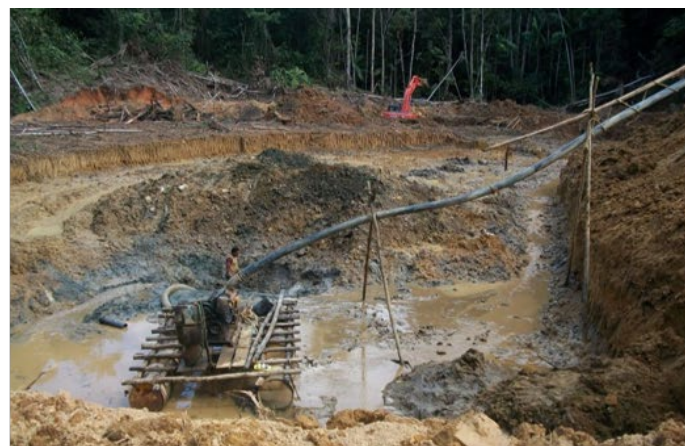
Figure 6 – Artisanal pit workings on the Gonini Project [circa 2019] (left) pit in saprolite exposing coarse quartz-rich gravels; (right) small-scale pump-and-sluice operation on the pit floor.
