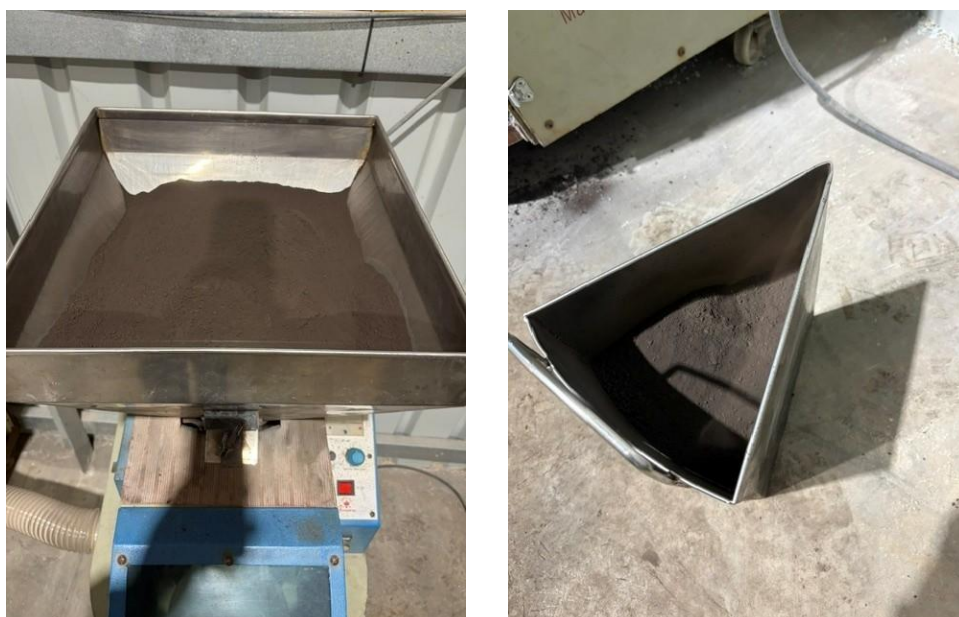
Figure 1. Milled Oakover manganese ore prepared as first feedstock for the ADP.
