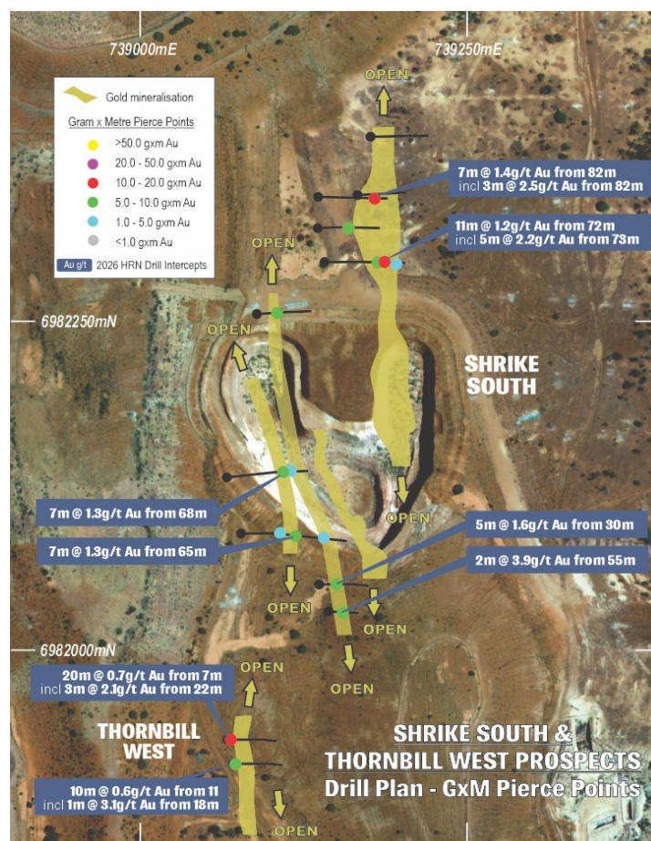
Figure 11: Shrike South & Thornbill West drill hole plan showing recent drill intercepts (>6 GxM) & gram x metre pierce points over satellite image.
