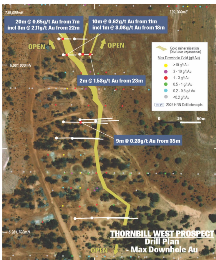
Figure 12: Thornbill Prospect drill hole location plan showing historic holes coloured by max. downhole gold and recent drill hole traces (white) and recent gold intercepts (labelled) over satellite image.
