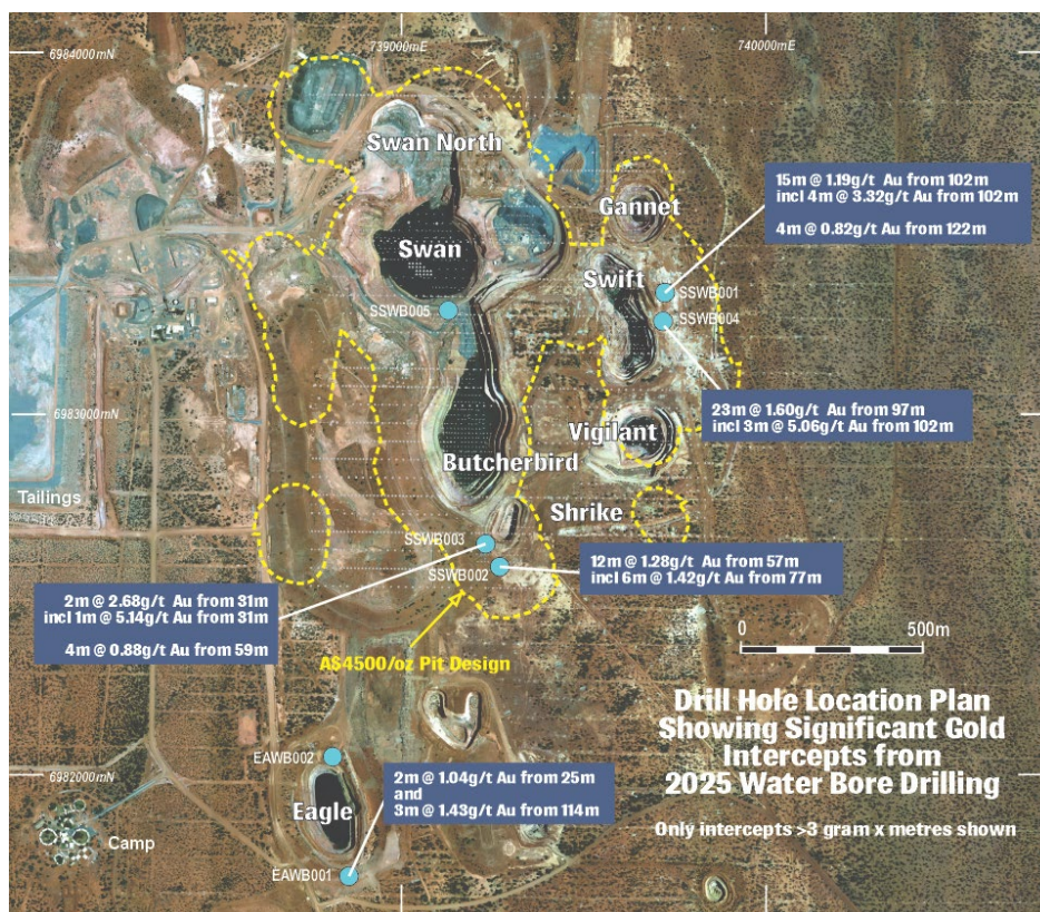
Figure 10: Swan-Swift Area water bore location plan showing A$4500/oz pit design outline, water bore collars (blue) and water bore gold intercepts >3 GxM (labelled) over satellite image.
