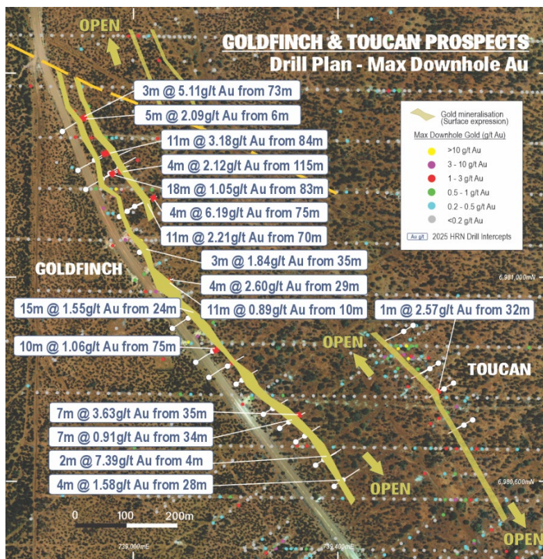
Figure 8: Goldfinch and Toucan Prospects drill hole location plan showing historic holes coloured by max. downhole gold, and recent drill hole traces (white) and selected recent gold intercepts >2.5 GxM labelled over satellite image.
