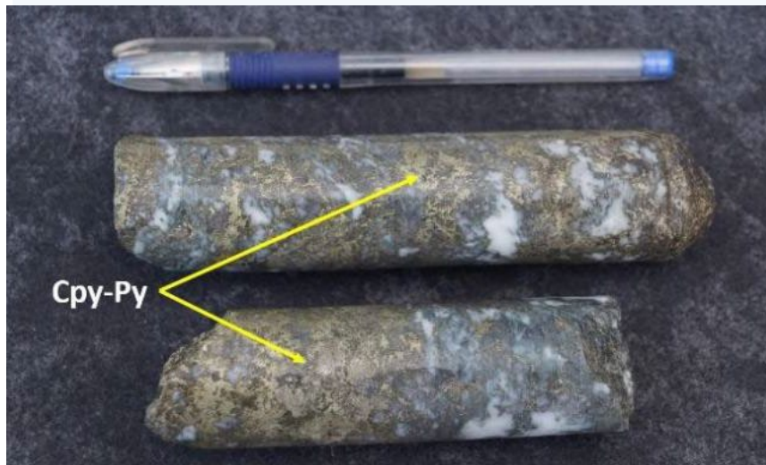
Quartz-chalcopyrite breccia mineralisation from 2022 short drill program, core CUL56-583 3 . This sample returned 8.0% Cu, 214 g/t Ag and 0.2 g/t Au . Drilling shows potential vein extension, located ~600m north of the Cutter Vein working 1
