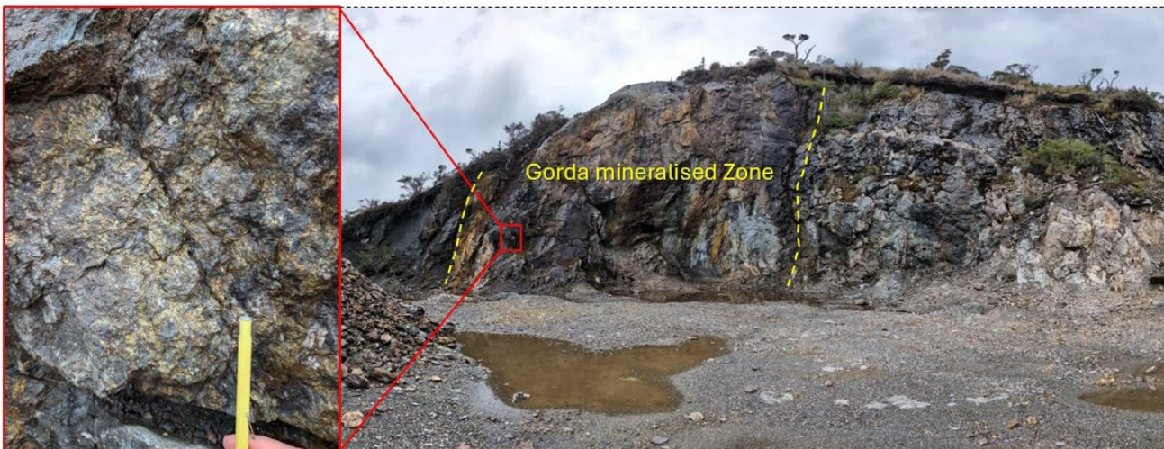
Quarry of the Gorda mineralised zone (~5m width), with insert showing chalcopyrite-quartz breccia hosted in Palaeozoic basement shale. Chalcopyrite estimate of 20% composition (Location 670,495m E, 4,085,504m N).
