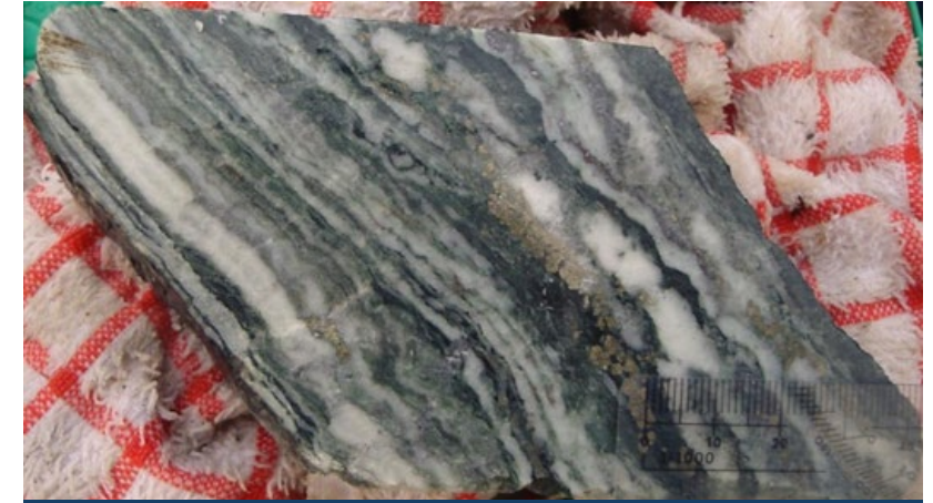
Crack-seal veining from the Gorda Vein , (25.31 m depth. Drillhole ZDD007 sample 898 (25.17m-26.17m): 8.25 ppm Au, 110 ppm Ag, 353 ppm Bi, 0.38% Cu. 1
