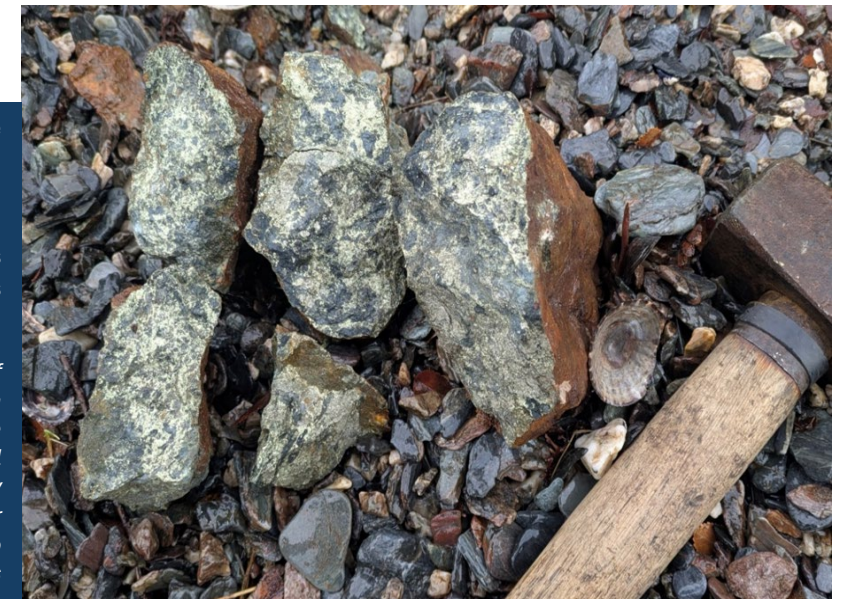
Crack-seal veining from the Gorda Vein , (25.31 m depth. Drillhole ZDD007 sample 898 (25.17m-26.17m): 8.25 ppm Au, 110 ppm Ag, 353 ppm Bi, 0.38% Cu. 1
