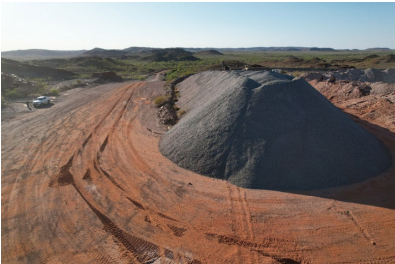
Figure 2: Commercial scale waste rock to road base trial product
