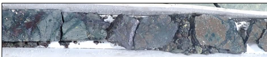
Figure 1. Core from GV-26-008 from 66.8 to 67.2m down hole, showing a highly altered breccia zone hosting silver-rich sulphide mineralisation. This interval returned 1.0m at 4,120g/t Ag, 5.7% Zn & 4.1% Pb from 66.7m.
