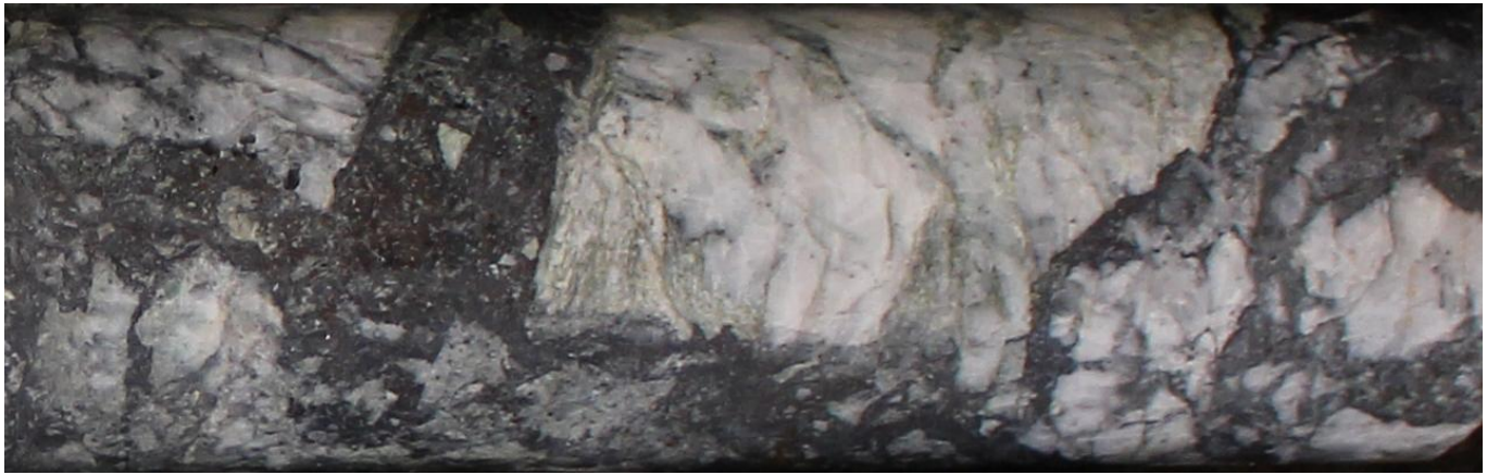
Figure 6 - BAR050 at metre 21.1 (5.2 g/t AuEq)
