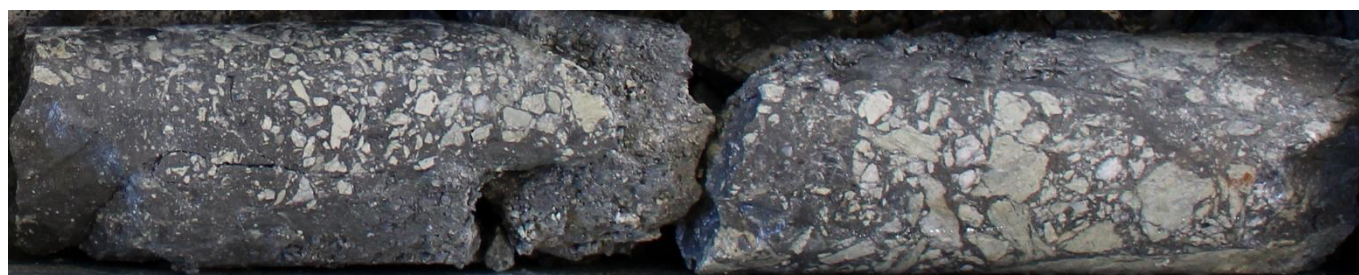
Figure 5 - BAR046 at metre 63.5 (15.7 g/t AuEq)
