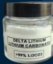
Figure 8: MT Ida Lithium carbonate produced from mica concentrate
