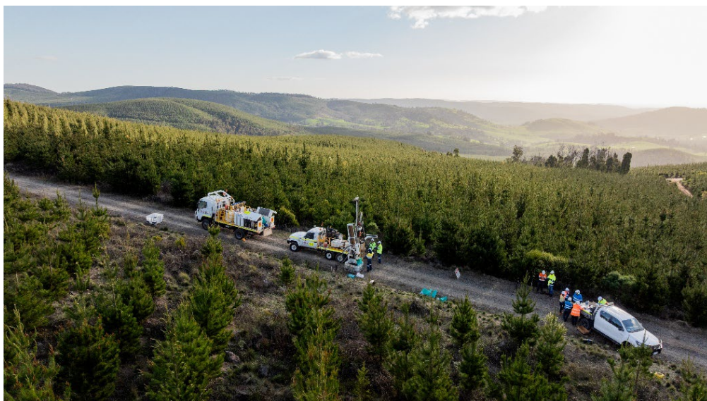
Figure 1: Aircore drill rig mobilised at the Blue Prospect within an FCNSW softwood plantation.
