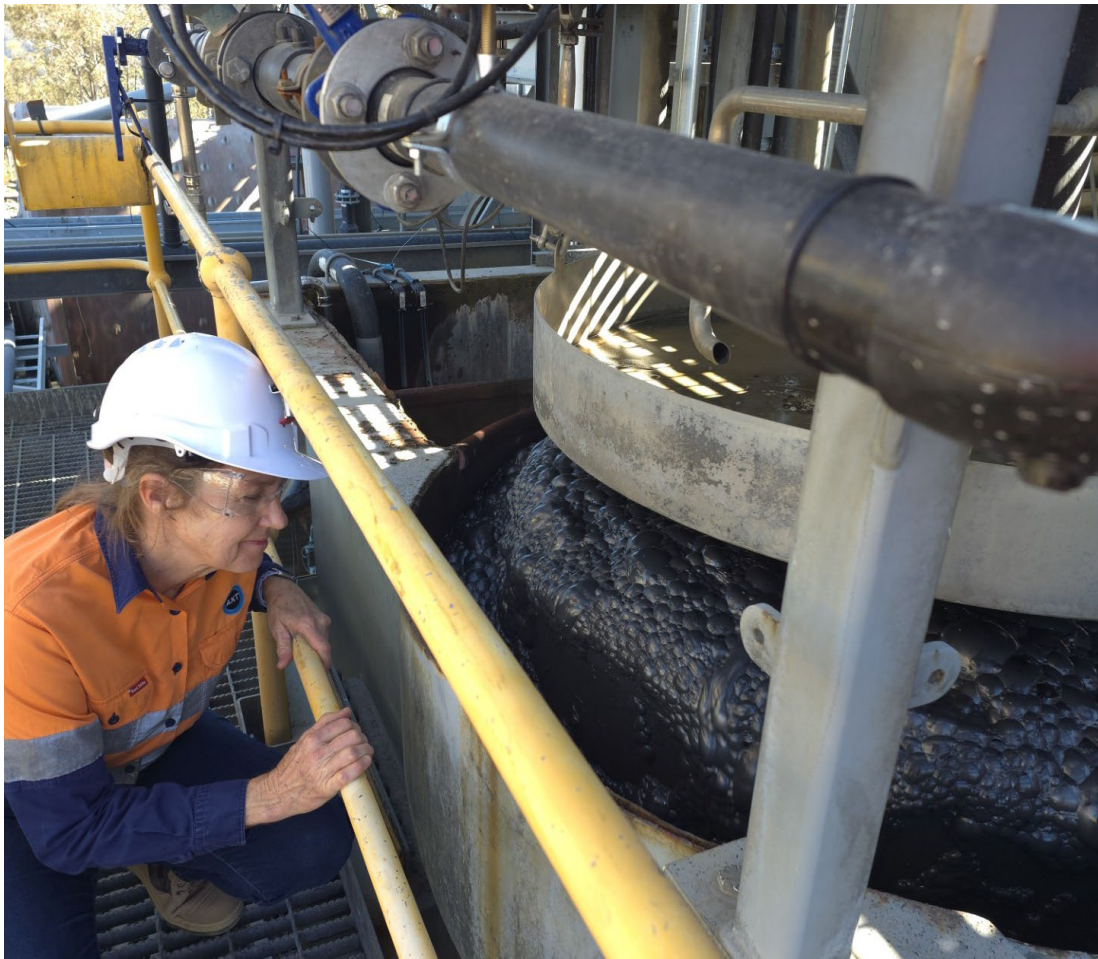
Figure 2 Jameson cleaner cell removing further impurities
