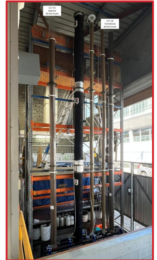
6m columns leach testing in progress
