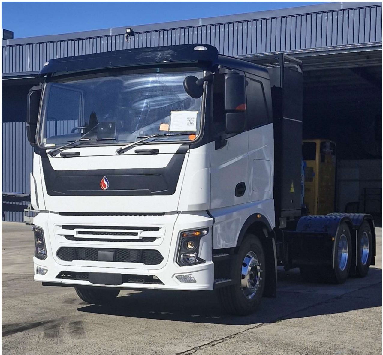
Right-hand drive battery swap prime mover Alpha by Pure One
