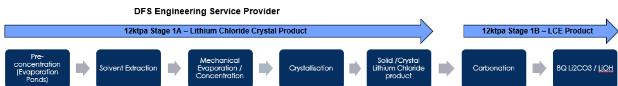
Figure 1. Rincon Lithium Project – Process Flowsheet
