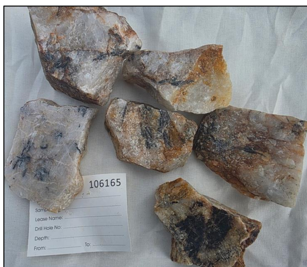
Figure 4. Sample No. 106165, milky white vein quartz with abundant coarse wolframite blades to 3 centimetres; assay result 5.5% W. (FOV 15 cms)
