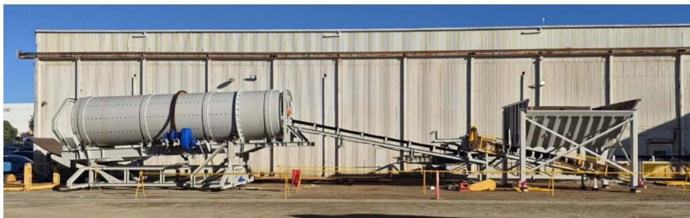
Figure 6: OZM feed bin, feed conveyor and agglomerator drum at Polaris Engineering Services Henderson Facility
