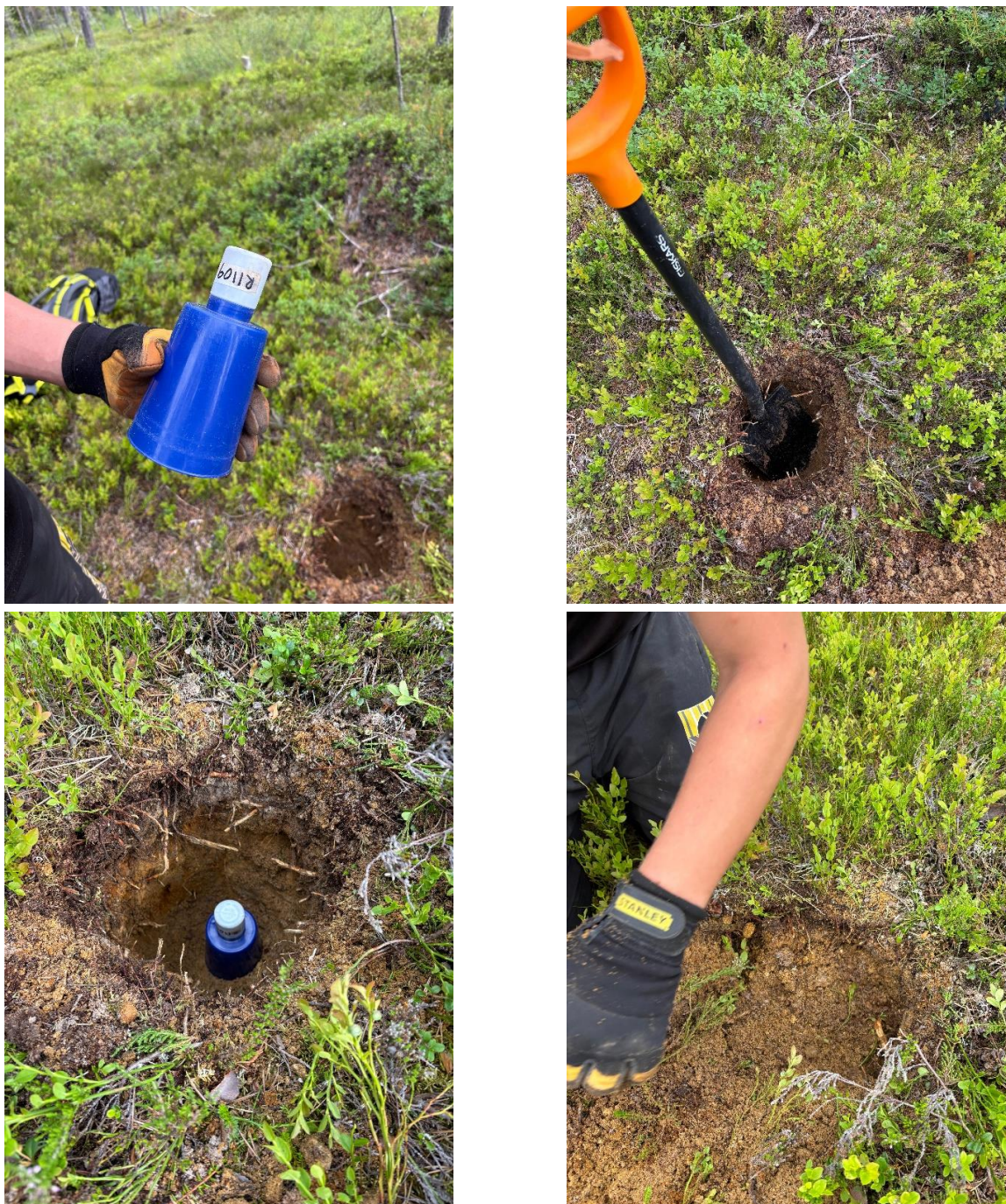
Figure 3: RadonX™ field deployment. Each inverted detector cup was buried in a shallow hole, its location recorded by GPS and marked with flagging tape, and recovered approximately 10 days later for field analysis.
