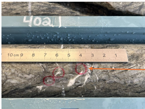
Image 1: 26FRD001 core at approximately 122.45–122.55m downhole showing red-circled visible native gold associated with quartz-feldspar-carbonate veining and pyrite mineralisation. Scale shown in centimetres and millimetres.
