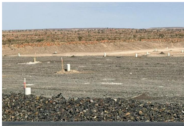
Future production areas drilled and cased
