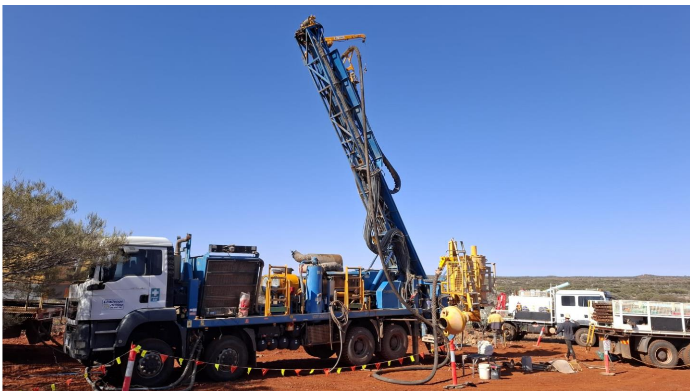
Figure 1: RC drilling underway at the Rochefort Gold Prospect, Abbotts North
