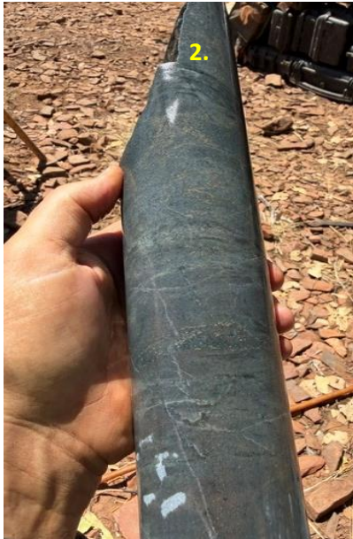
Photo 1 - 3: Grey metamorphosed sandstone with silica/sericite alteration with disseminated brassy pyrite throughout (1 - 5% Pyrite) with quartz carbonate bands (36.6m to 40.3m – BDDD002).
