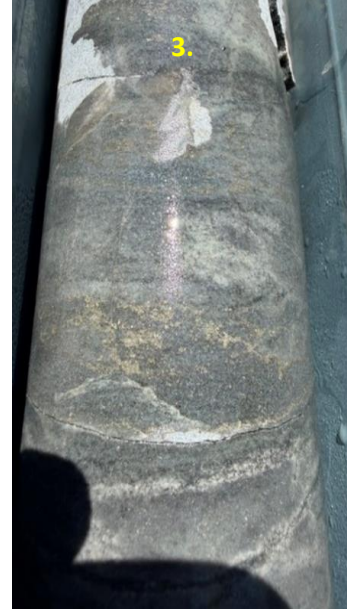
Photo 1 - 3: Grey metamorphosed sandstone with silica/sericite alteration with disseminated brassy pyrite throughout (1 - 5% Pyrite) with quartz carbonate bands (36.6m to 40.3m – BDDD002).
