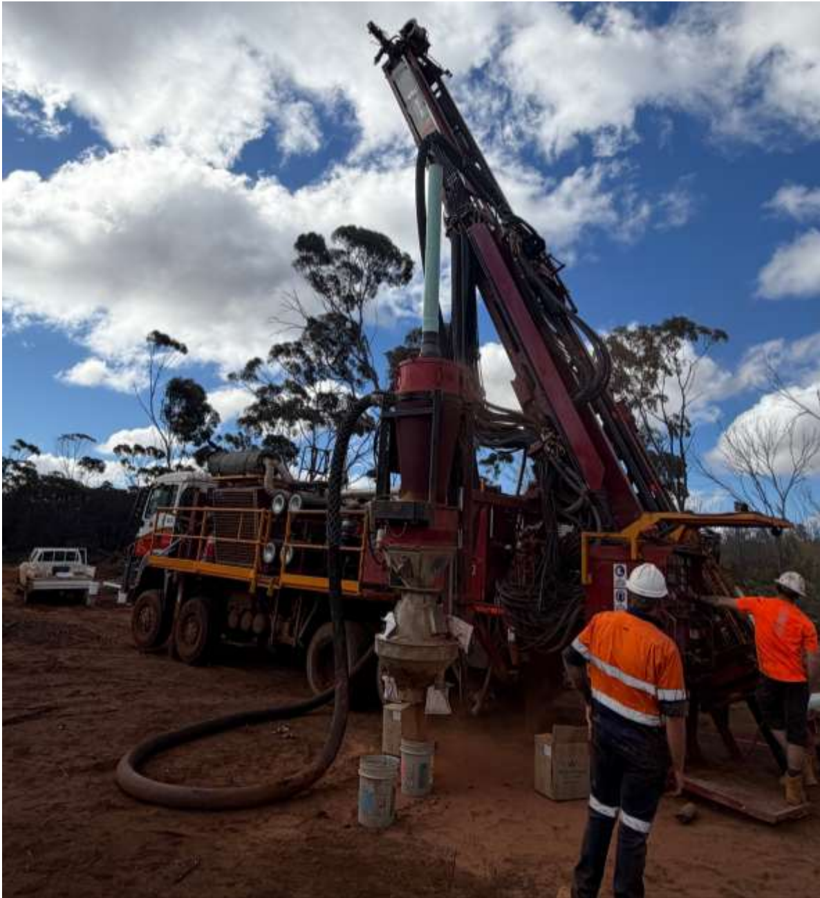
Photo 1. VM Drilling's RC Rig: drilling underway at Medcalf Spodumene Deposit.
