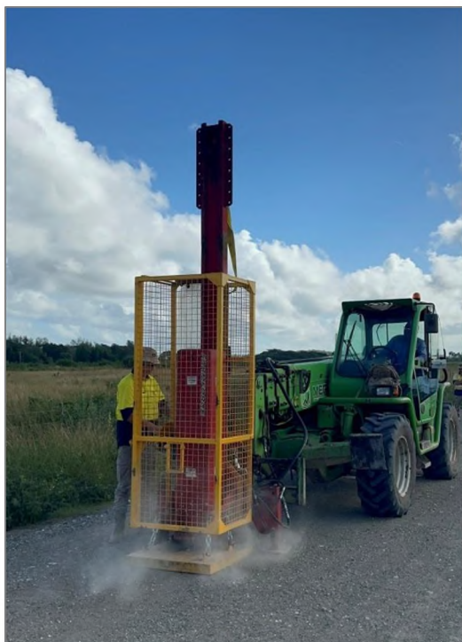
Figure 4 – “Thumper” weight-drop system in action
