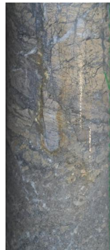
NSD058 – 283.5m. Basalt-proximal, carbonate-silica altered, brecciated and annealed unit with disseminated acicular arsenopyrite throughout.
