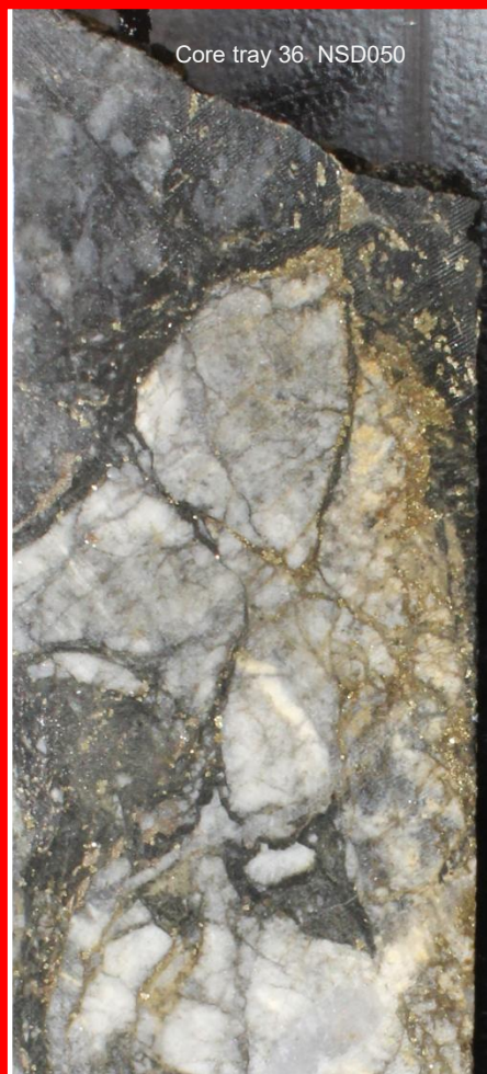
NSD050 illustrating carbonate-quartz vein crosscutting earlier carbonate and chloritic domains
