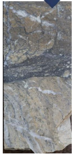
NSD058 – ~283.5m the intercept, although narrow, includes very encouraging geology and structure that indicates the possibility of a Stawell-type gold system.
