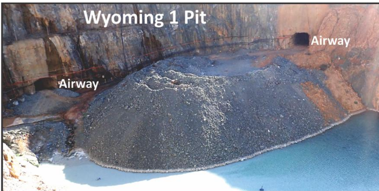
Figure 16-6: Additional airways in the Wyoming Pit
