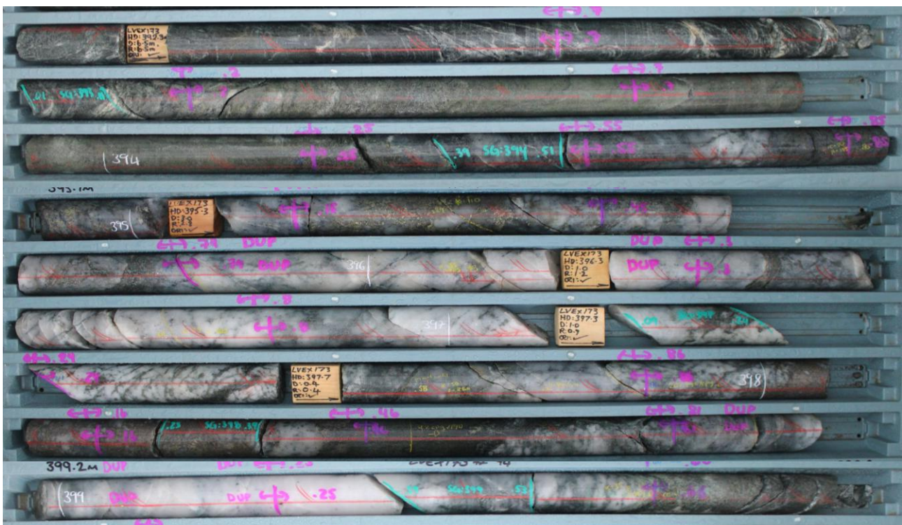
Figure 4. Core photo of LVEX173 showing mineralised intercept from 392.7m, 7.0m @ 12.6 g/t Au
