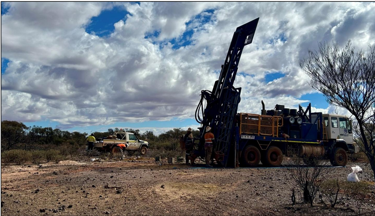
Figure 10: Air core drilling at the Diorama Copper-Gold Target.
