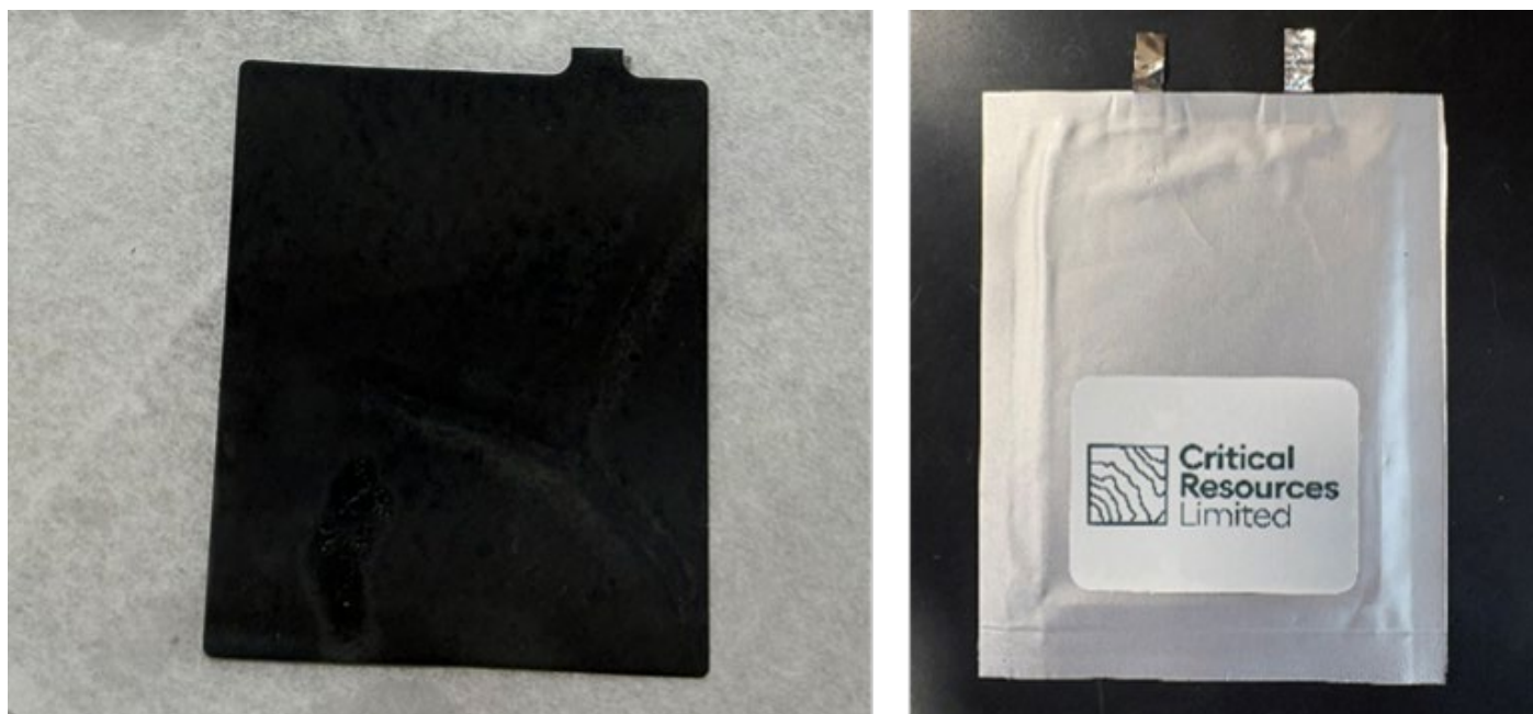
Figure 3 – LEFT – Post-test inspection of the cell: the lithium-metal anode shows heavy degradation, consistent with reaction with the liquid electrolyte, while the DSD-deposited cathode appears stable and intact on visual inspection. RIGHT – The full-format test cell.
