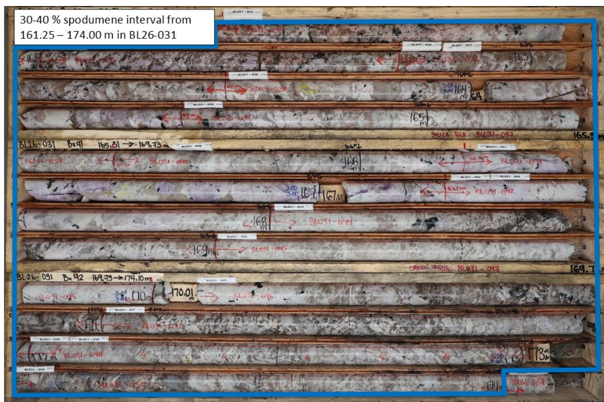
Figure 4: Spodumene pegmatite with visual estimates of 30-40 % spodumene from 161.25 – 174.00 m within larger interval that averages 15-25% spodumene based on visual estimates in drill hole BL26-031. 1
