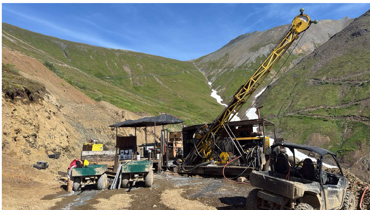
Figure 4. Diamond drill rig producing oriented diamond core at Caribou Dome
