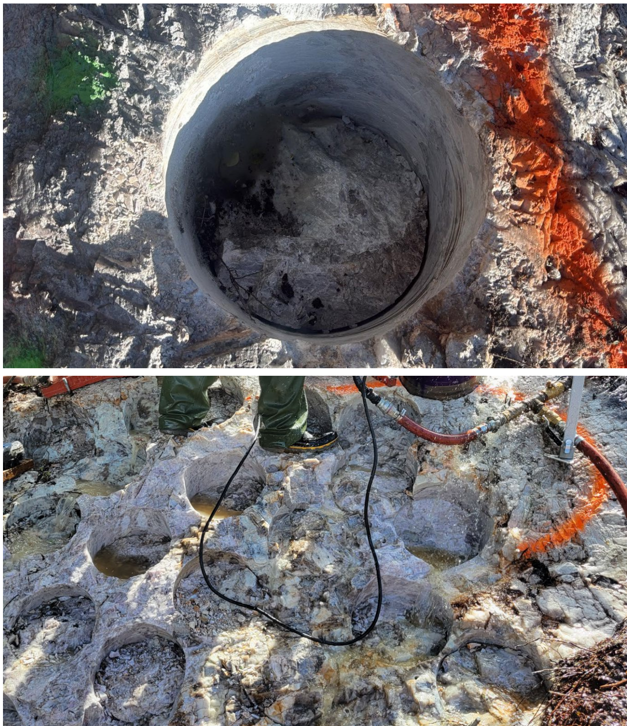
Figure 2: (TOP) Cored drill hole (~30 cm diameter) in pollucite pegmatite outcrop; (BOTTOM) Grid of cored drill holes (~30 cm diameter) in pollucite pegmatite outcrop (see Table I). Segments between holes are jackhammered out and added to sample composite.
