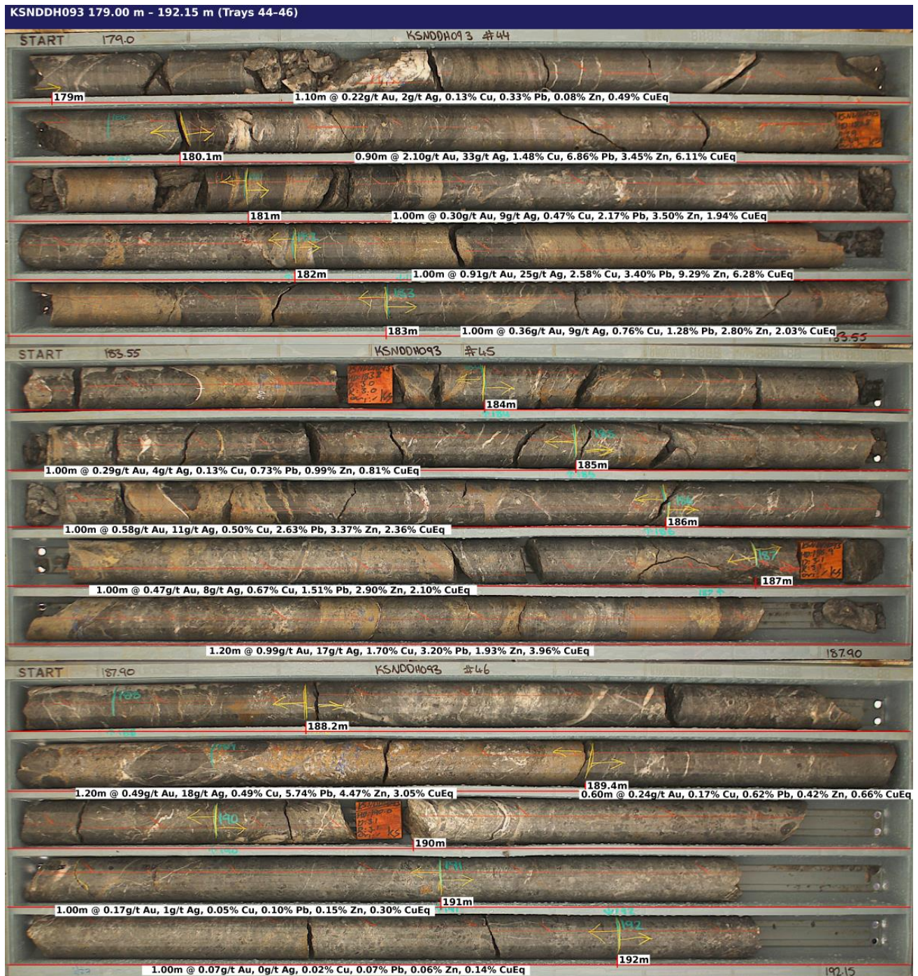
Figure 5: Core photos KSNDDH093, 179m - 192.15m, showing chalcopyrite, galena, sphalerite mineralisation.
