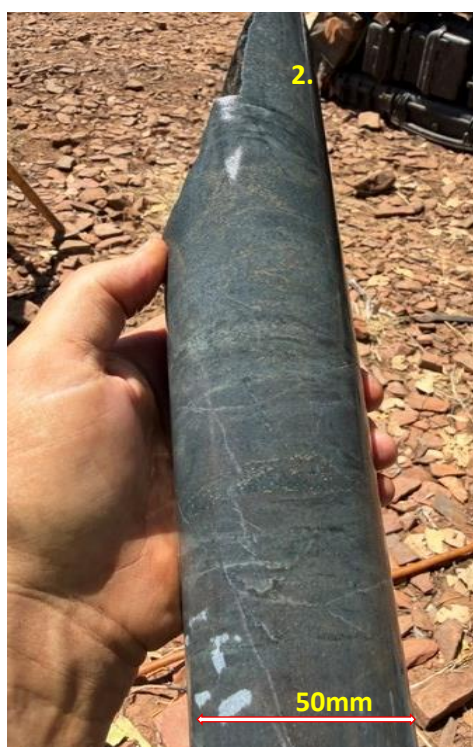
Photos 1 to 4: Grey metamorphosed sandstone with silica/sericite alteration with disseminated brassy pyrite throughout (1 - 5% Pyrite) with quartz carbonate bands (36.6m to 40.3m – BDDD002).
