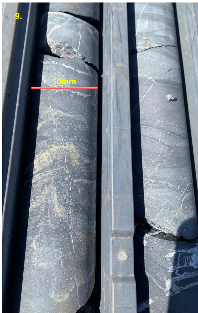
Photo 9 & 10: Pyrite bands and carbonate veinlets in black shale (399m – BDDD002).
