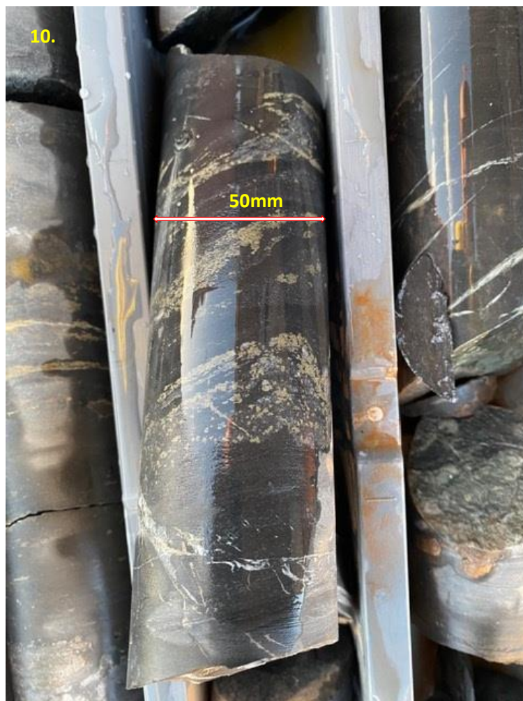
Photo 9 & 10: Pyrite bands and carbonate veinlets in black shale (399m – BDDD002).
