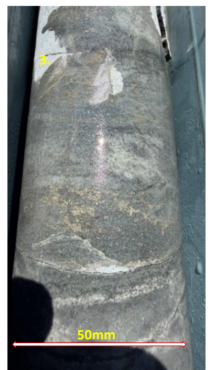
Photos 1 to 4: Grey metamorphosed sandstone with silica/sericite alteration with disseminated brassy pyrite throughout (1 - 5% Pyrite) with quartz carbonate bands (36.6m to 40.3m – BDDD002).
