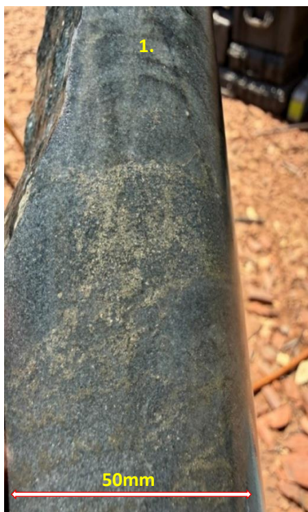
Photos 1 to 4: Grey metamorphosed sandstone with silica/sericite alteration with disseminated brassy pyrite throughout (1 - 5% Pyrite) with quartz carbonate bands (36.6m to 40.3m – BDDD002).
