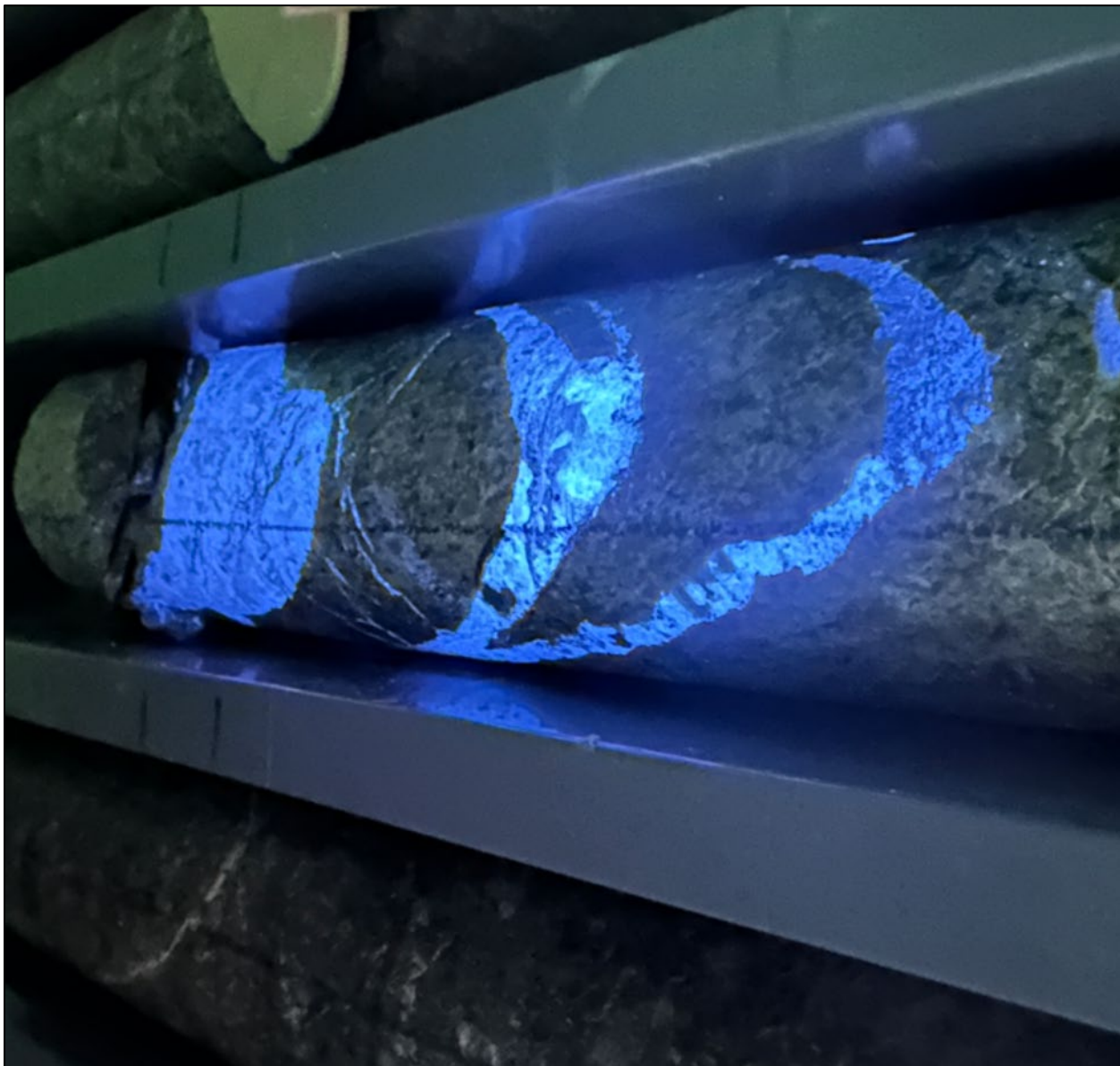
Figure 4 High-grade tungsten-bearing scheelite mineralisation in drillhole CLG129 under UV light, returning 1m @ 7.27% WO 3 from 375m.
