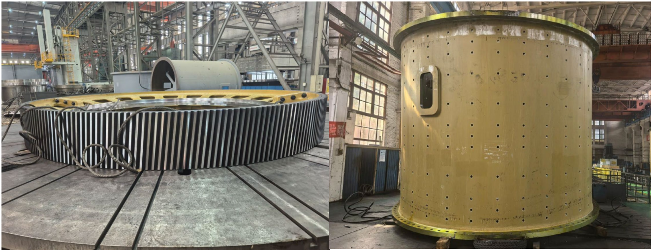
Figure 7 – Ball Mill girth gear and 1 of 2 shells
