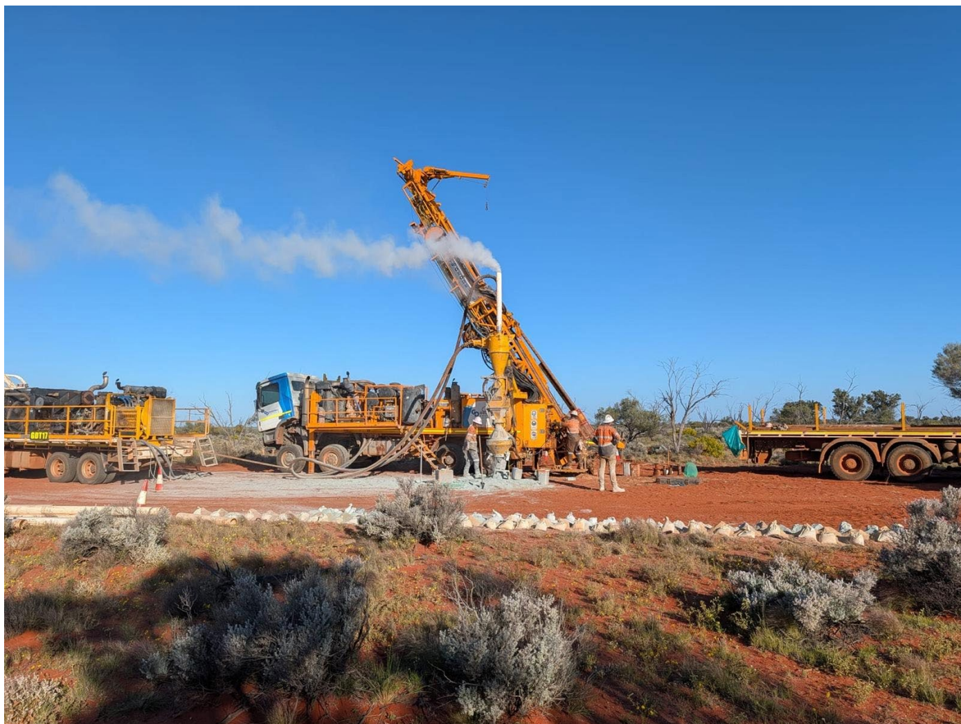
Figure 1: RC drilling first hole at Company Well.
