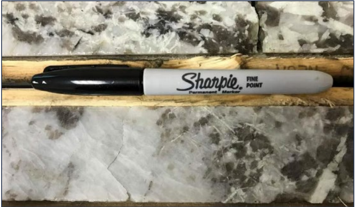
Figure 7-9: Coarse to Fine-Grained Spodumene Mineralization in Hole NAL-16-024
