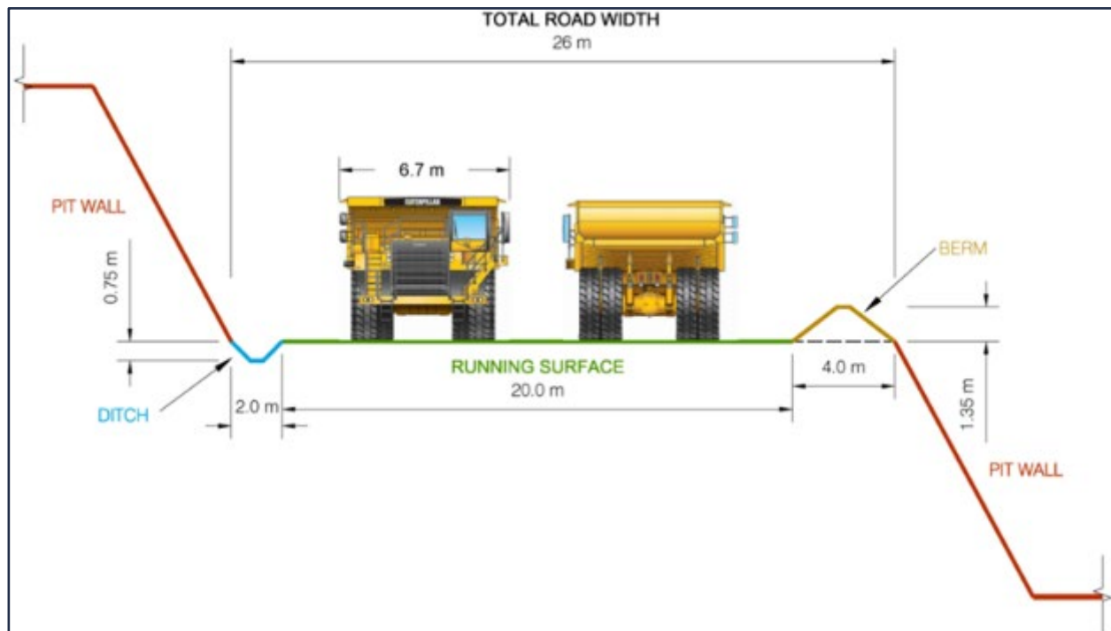
Figure 16-6: Dual-Lane in-Pit Haul Ramp Design
