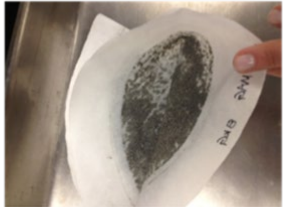
Figure 13-5: Magnetic and Non-Magnetic Fractions from Test Conducted at 8,000 Gauss
