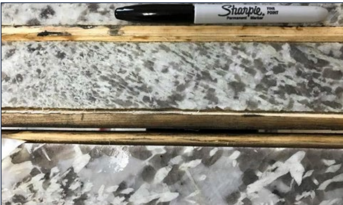
Figure 7-7: Preferential Orientation of Spodumene Crystals in Hole NAL-16-024
