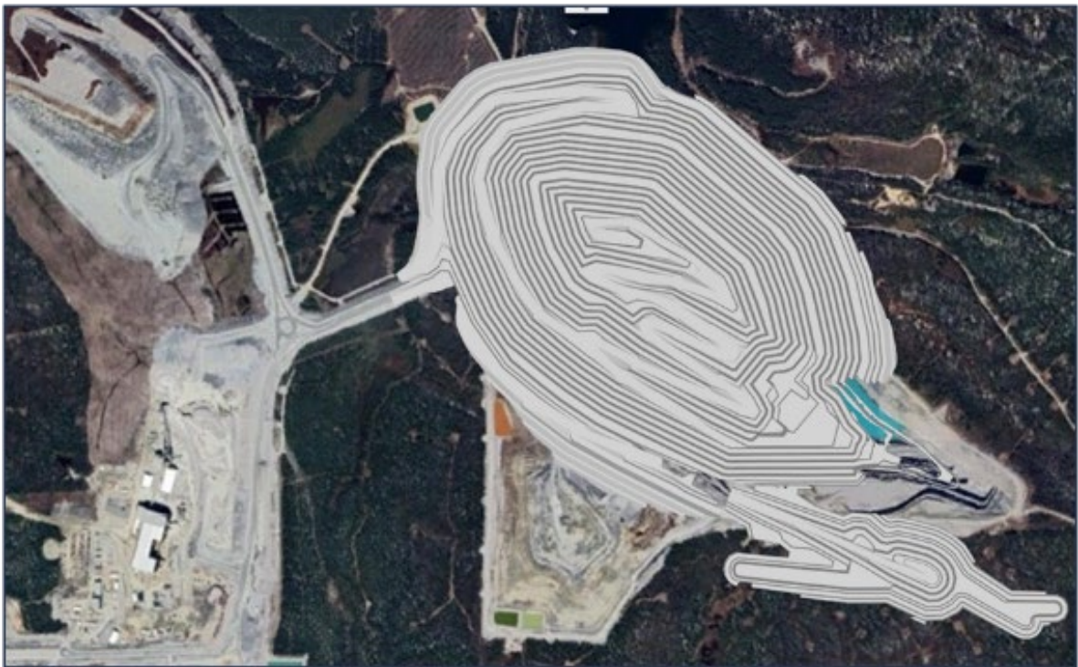
Figure 16-1: NAL Final Pit Design
