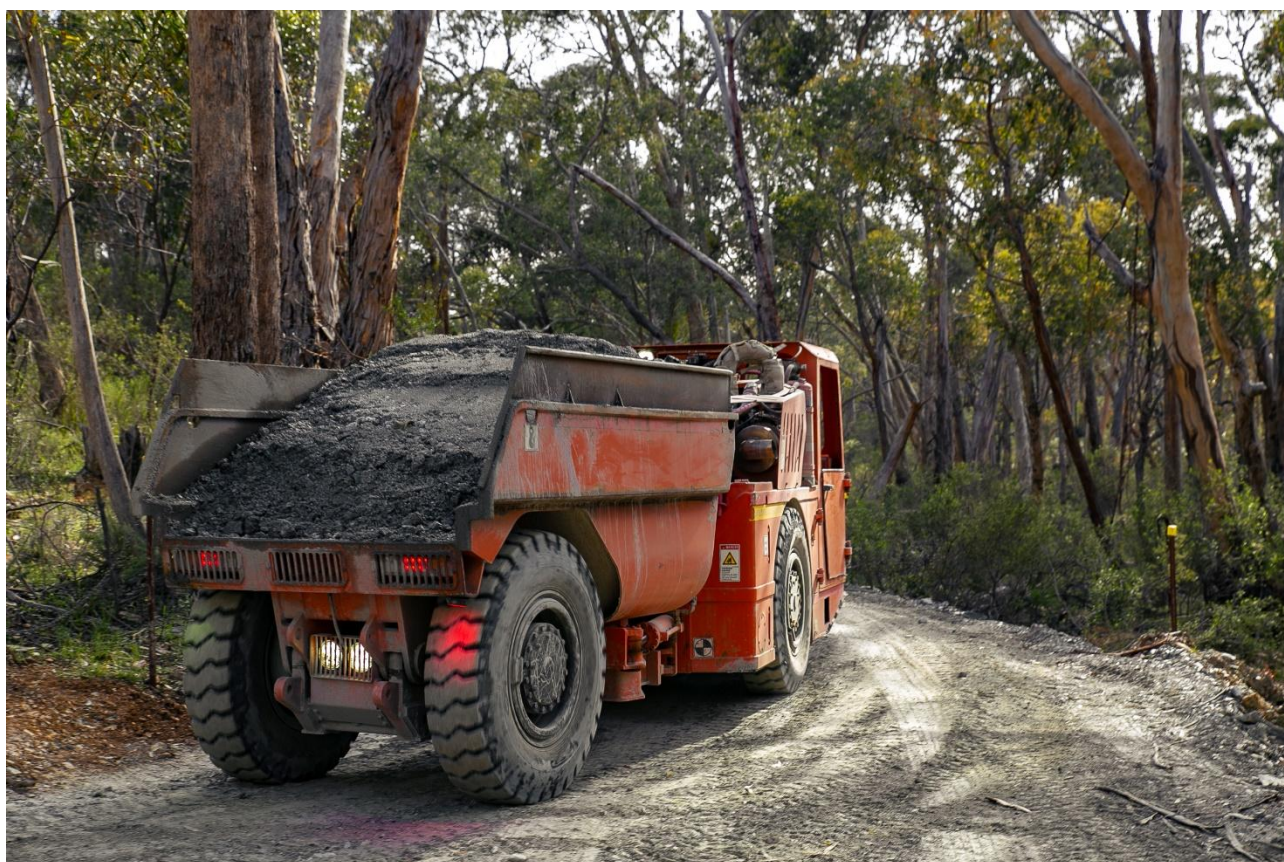
Figure 2 – Haul truck carting ore at the Fiddlers Creek high grade gold and silver underground mine.
