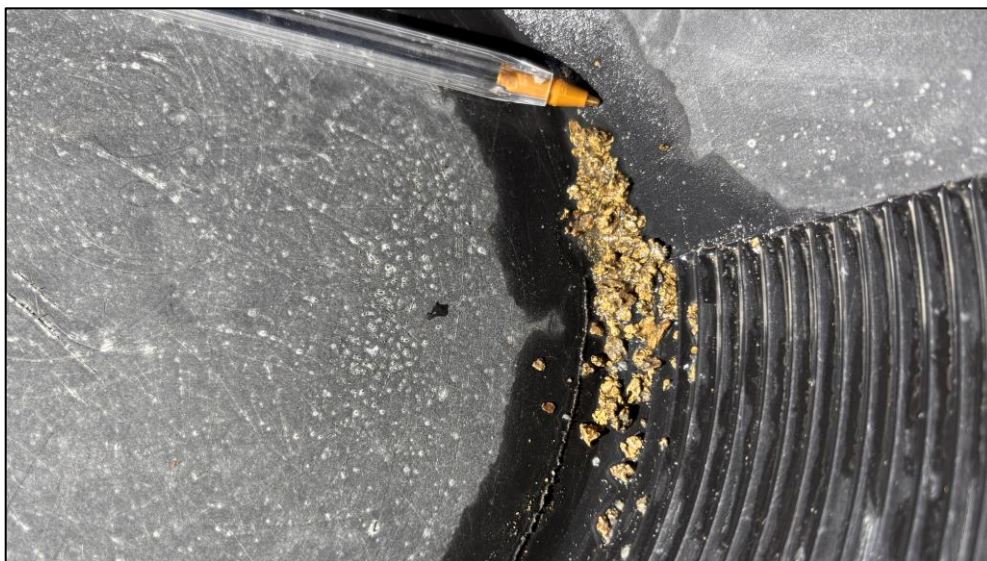
Figure 2: Gold nuggets produced from RC drillhole BORC26036, 202-203m, which produced an intercept of 1m @ 751g/t Au, within a broader intercept of 7m @ 119g/t Au from 199m
