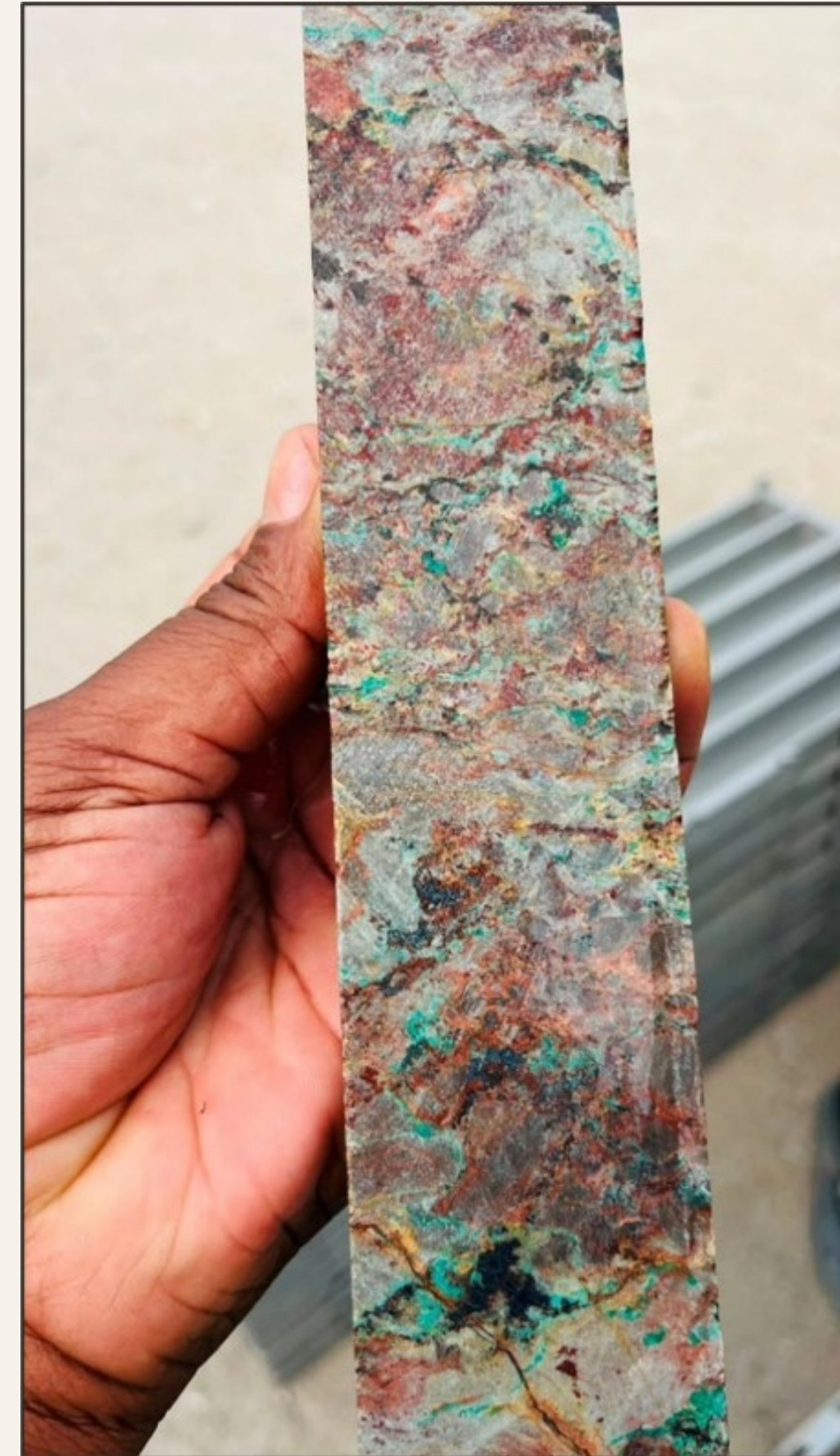
DDOT002 Core from 68.13m to 68.34m showing disseminated malachite, chrysocolla, cuprite and chalcocite mineralisation 1 (left) and DDOT001 Core from 64.03m to 64.17m showing disseminated chalcocite, cuprite and diopside mineralisation (right).
