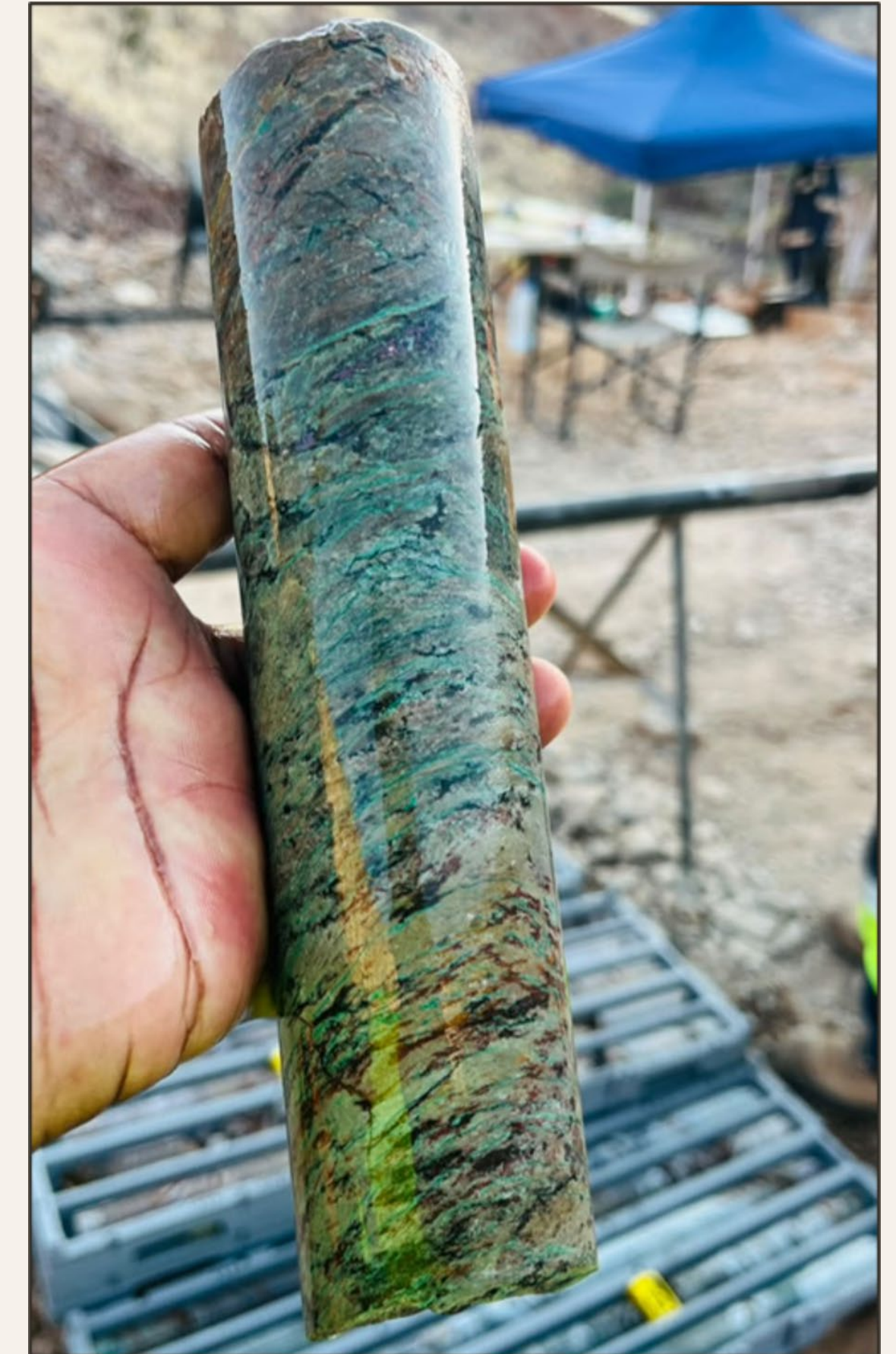
DDOT002 Core from 68.13m to 68.34m showing disseminated malachite, chrysocolla, cuprite and chalcocite mineralisation 1 (left) and DDOT001 Core from 64.03m to 64.17m showing disseminated chalcocite, cuprite and diopside mineralisation (right).
