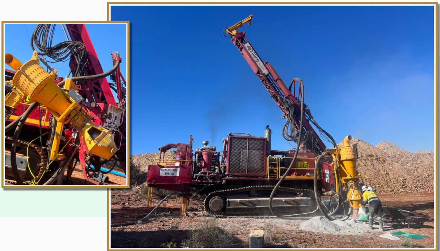
Picture 1,2: Track mounted RC drill rig for the program (shown at latest Golden Crown drilling).
